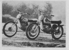
All three bikes have aluminum alloy wheels. The Honda has redesigned lighter DIDs. The YZ has Takasagos; the MX has DIDs. All three bikes have two rimlocks on the rear. Both Yamahas have two locks up front, Honda only has one. Wheels on all three bikes shed mud.
