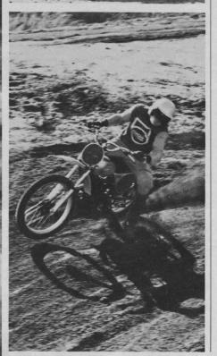
comes fitted with only a 3.50 sized tire. The machine is quite capable of pulling a four incher, and this would help it hang in there more on the corners.
